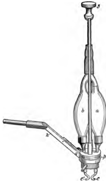
Fig. 177.—Ludwig's stromuhr: a and b , the glass bulbs; a is filled with oil to the mark (5 c.c.), while b and the neck are filled with salt solution or defibrinated blood; p , the movable plate by means of which the bulbs may be turned through 180 degrees, c, c , for the cannulas inserted into the artery; s , the thumb screw for turning the bulbs; h , the holder. When in place the clamps on the arteries are removed, blood flows through c into a , driving out the oil and forcing the salt solution in b into the head end of the artery through c' . When the blood entering a reaches the mark, the bulbs are turned through 180 degrees so that b lies over c . The blood flows into b and drives the oil back into a . When it just fills this bulb, they are again rotated through 180 degrees, and so on. The oil is driven out of and into a a given number of times, each movement being equal to an outflow of 5 c.c. of blood. When the instrument has been turned, say, ten times, 50 c.c. of blood have flowed out. Knowing the time and the caliber of the artery, the calculation is made as described in the text. A modification of the form of this instrument has been devised by Tigerstedt.*
